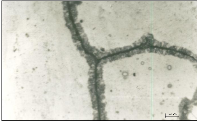
Fig.1. Structural evolution of Ni-1,4 at % In alloy, after homogenization at 1048°C during 400h, quenched in ice water and annealing at 600°C during 3h
