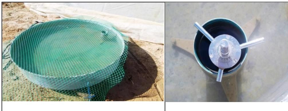
Figure 01: "Class A" evaporation pan(left) and level gauge (right)
